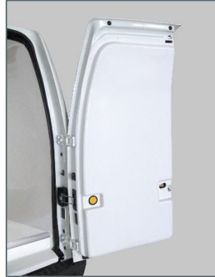
Rear door with molded insulated fiberglass cover.
