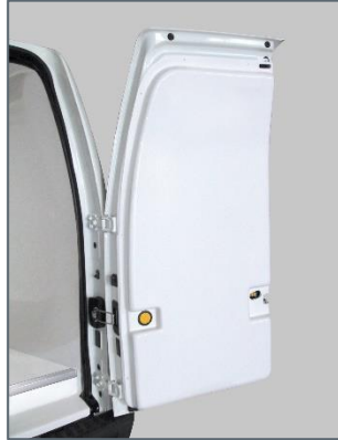
Rear door with molded insulated fiberglass cover.
