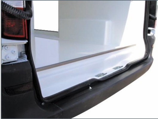
Edged floor to avoid water leak. Stainless steel threshold.
